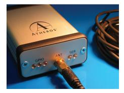
Complete with software and an integrated AR1511 daughterboard, the AR1511 Evaluation Kit (EVK) is a full-featured GPS receiver that provides a conventional platform to evaluate the performance of the AR1511 and Orion software.
