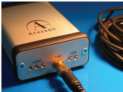
Complete with software and an integrated uN3010 daughterboard, the ORION RX2 Evaluation Kit (EVK) is a full-featured GPS receiver that provides a conventional platform to evaluate the performance of the ORION RX2™.
